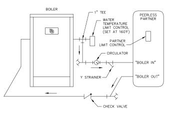
Figure 4.5: Typical Steam Boiler Indirect Water Heater Piping
