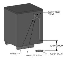
Figure 6.6: Relief Valve Piping Water Boiler
