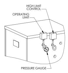
Figure 6.5: Limit Control Installation
