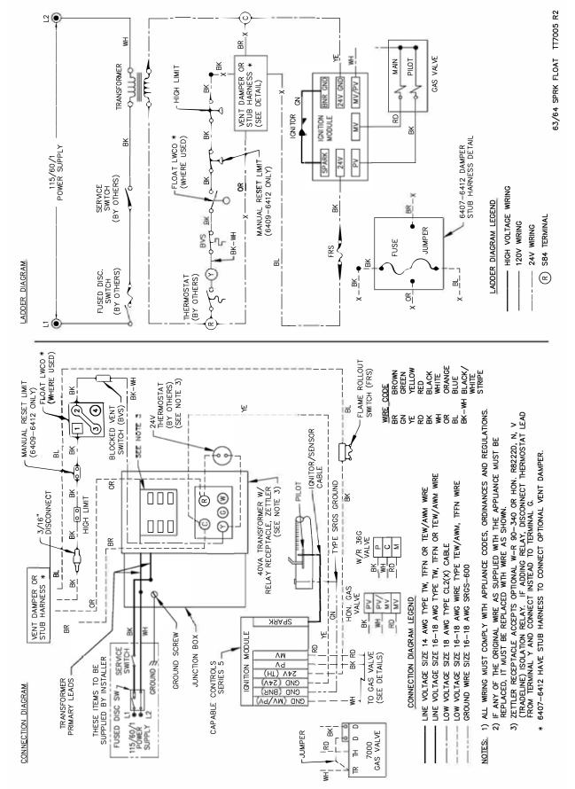
Figure 7.5: Steam Boiler – Wiring Diagram for Models with Float Low Water Cut-off
