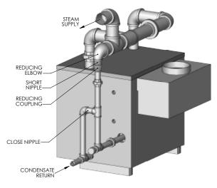
Figure 4.4: Steam Piping – Dual Supply Connections
