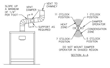
Figure 3.3: Venting with Vent Damper in Horizontal Position
