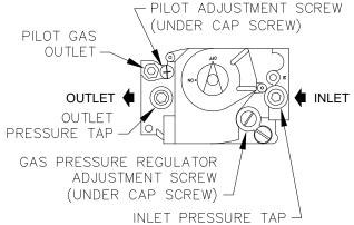
Figure 5.5: Valve Tapping and Adjustment Screw Locations, Honeywell
