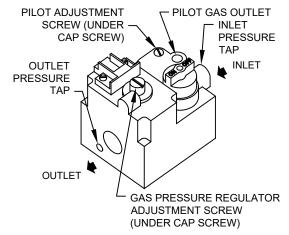
Figure 5.7: Valve Tapping and Adjustment Screw Locations, Robershaw 7000
