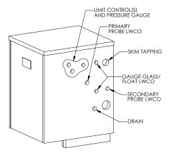
Figure 6.2: Steam Boiler Tapping Location
