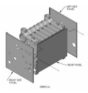
Figure 2.5: Jacket Assembly, Series 64™ Boilers
