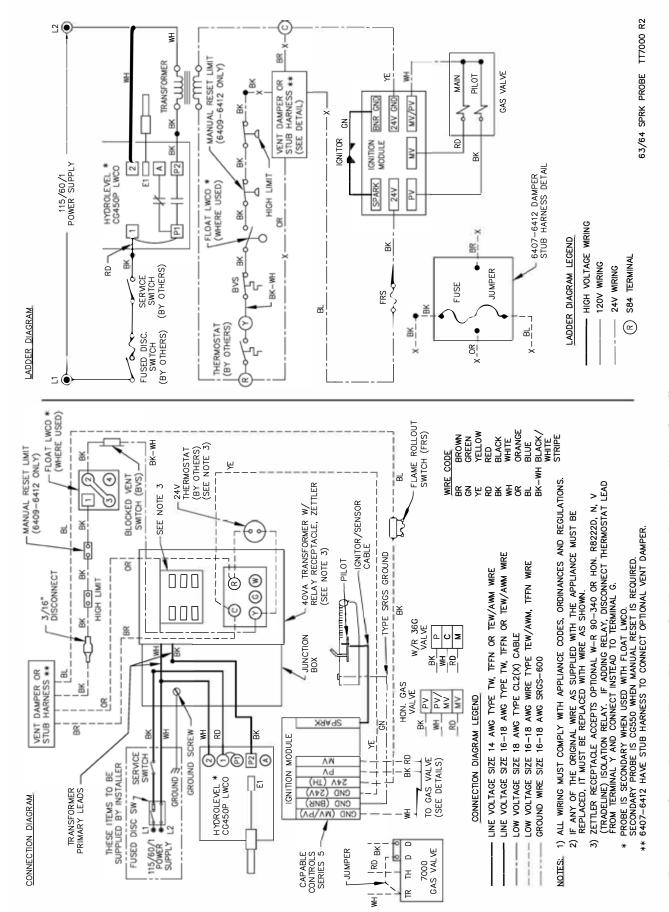
Figure 7.6: Steam Boiler – Wiring Diagram for Models with Probe Low Water Cut-off
