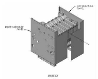
4. **Back Panel Jacket:** Position the back jacket panel inside the flange of the side jacket panels and attach it with six #10 x 1/2" sheet metal screws. See Figure 2.5.
