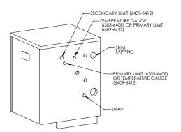
Figure 6.7: Water Boiler Tapping Locations
