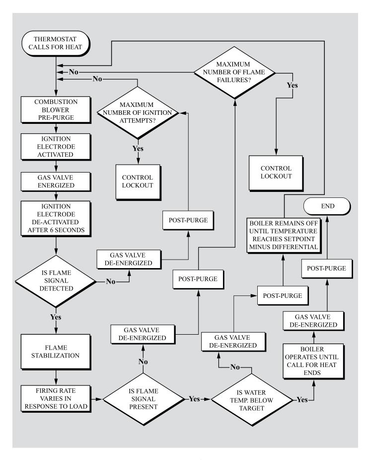
Figure 5: Sequence of Operation
