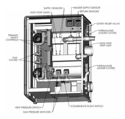
Figure 2: Control & Safety Device Locations – PFC-850/1000/1500
