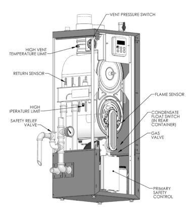
Figure 1: Control & Safety Device Locations - PFC-460
