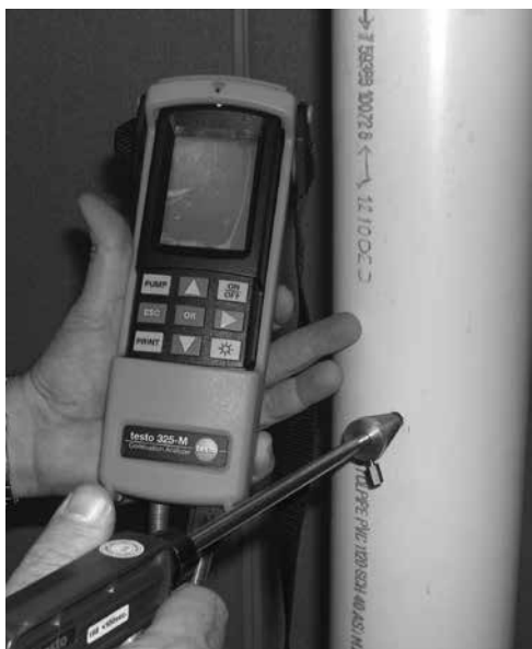
Figure 9.2: Insert Analyzer Test Probe into Test Port
