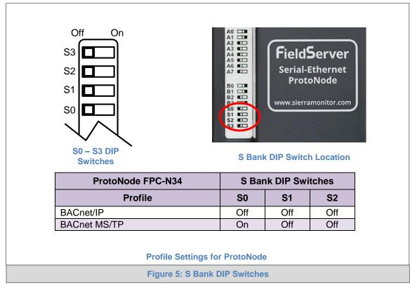
**NOTE:** When setting DIP Switches, ensure that power to the board is OFF.
