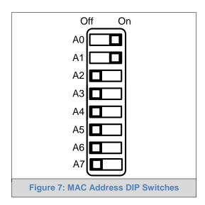
**NOTE:** When setting DIP Switches, ensure that power to the board is OFF.
